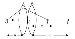
An object is placed at point *O*. The lens *A* produces an image at  $I_1$  which serves as a virtual object for lens *B* which produces final image at *I*.
