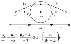
Note that the real image is formed only when the refractive index of the sphere is more than that of the surrounding, *i.e.*,  $\mu_2 > \mu_1$ .
